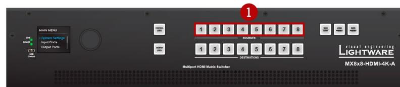
If every source, destination, and **Take** buttons are unlit (the unit is in **Take** mode, and no input was selected in the last 3 seconds), press and release a **destination button** to see its current state. Now the source button, which is connected to the selected destination, will light up.
