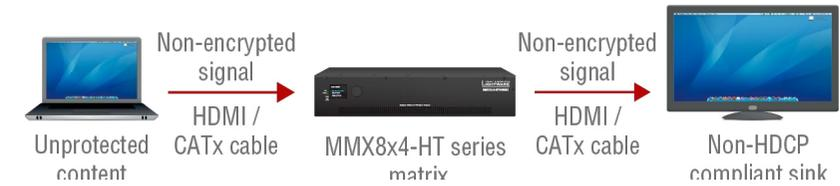
Not-HDCP compliant sink is connected to the matrix. Some sources (e.g. computers) always send HDCP encrypted signals if the receiver device reports HDCP compliancy, however, HDCP encryption is not required all the time (e.g. computer desktop image). If HDCP is enabled in the matrix, the image will not be displayed on the sink.
