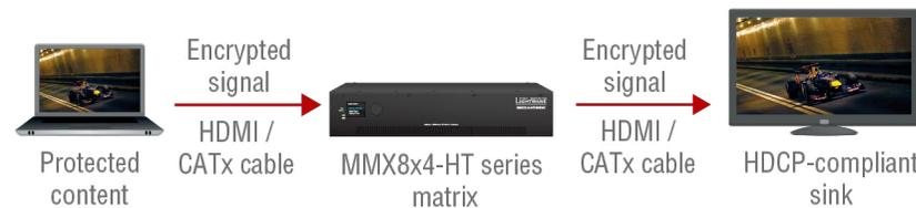
All the devices are HDCP-compliant, no manual setting is required, both protected and unprotected contents are transmitted and displayed on the sink.
