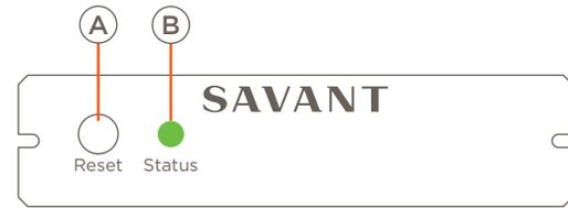
**Press** will place the device in remote pairing mode, this will turn the Status LED red.
