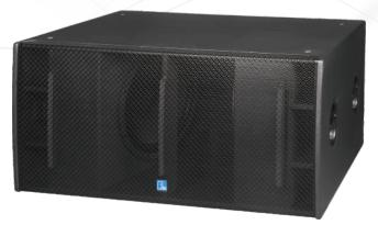
**DLA218B** is a dual 18" subwoofer. It features 2x18" 100mm voice coil woofer,bass-reflex design, can be used with line array and point source full range speakers to improve the low frequency performance. The cabinet is made of multilayer composite plywood with wear-resistant polyurea paint.
