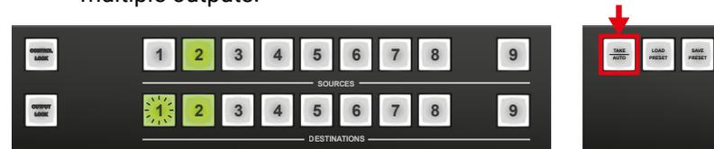
**ATTENTION!** A **source** button can be pressed twice to preselect all outputs. Outputs which are connected to the pressed input light up and all other outputs start to blink. Some outputs can be unselected if needed, and then pressing **Take** executes the switching.
