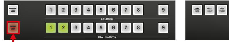
Now the **Output Lock** button starts to blink and the buttons of all the locked **outputs** illuminate green (view state). If no button is pressed for three seconds the router returns to idle state.
