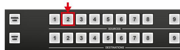
The pressed source button and all destination buttons which are currently connected to this source will light up.
