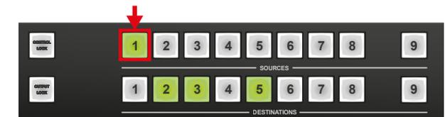
For viewing output connections, press and release a **destination** button. Now the source button which is connected to the selected destination will light up. If no source button is lighting, the selected destination is in muted state.
