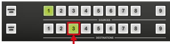
**ATTENTION!** Be careful, as if a **source** button is pressed in Autotake mode, it is immediately connected to the last selected destination.
