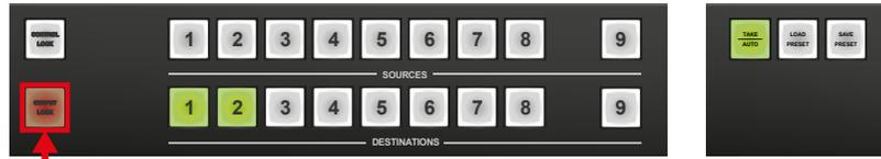
Now the **Output Lock** button lights up in red, and lock function is activated at once. No source can be changed at the locked destination.
