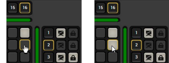
For example, input 16 is not connected to output 2 according to the first picture below. After the connection is established the square becomes light grey.
