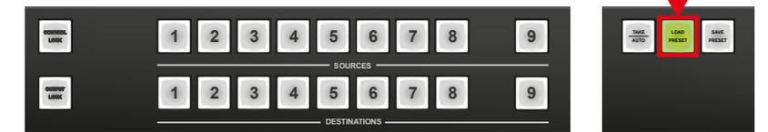
**Step 2.** Press and release a **source** button according to the desired memory address.
