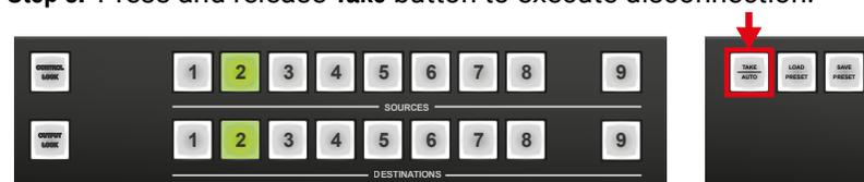
**INFO:** Deselected destinations are disconnected from any source, thus output devices will display black image or **no signal** message, or automatically will turn off.
