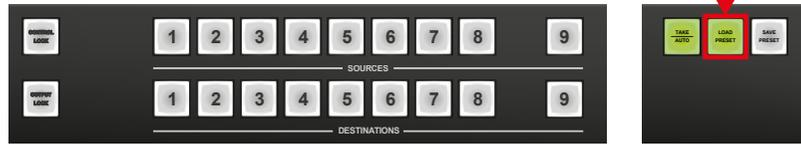
**Step 2.** Press and release a **source** button according to the desired memory address.
