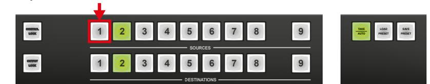
Switching is executed immediately. Switching between sources to the selected destination can be done directly.
