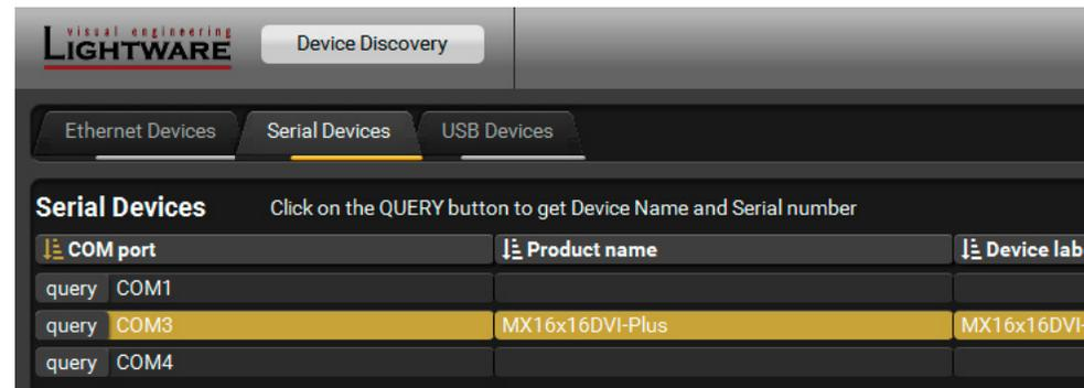
**ATTENTION!** When the device is connected via the local RS-232 port, make sure that LW protocol (#1) is set on the serial port. The protocol settings are available by the front panel buttons, see the [Control Protocols](#) section.
