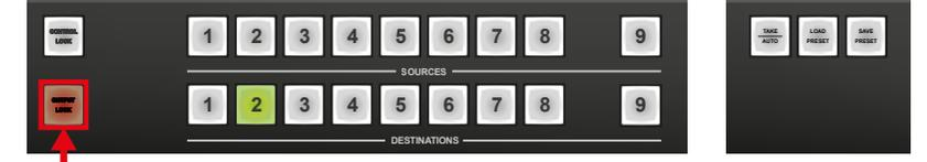
Now the **Output Lock** button starts to blink and all the locked output's buttons illuminate green (view state). If no button is pressed for three seconds, the router returns to idle state.
