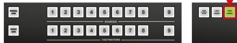
**Step 3.** Press and release a **source** button according to the desired memory address.
