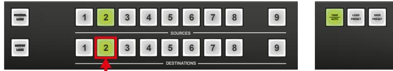
Now the selected destination button and the currently configured **source** button and the **Output Lock** button light up.
