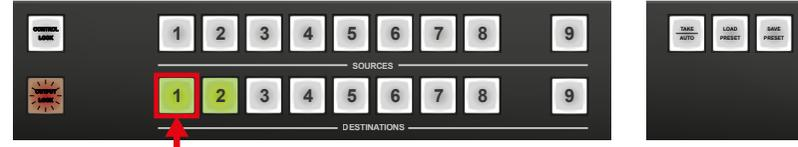
If an unlit output button is pressed it starts to blink indicating that it is preselected, for output locking.
