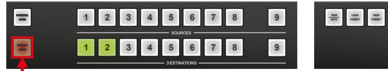
**Step 2.** The **Output Lock** button starts to blink and all the buttons of any locked destinations light up and remain illuminated for three seconds.
