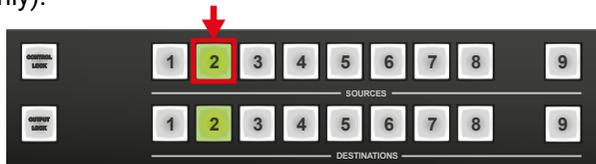
**Step 2.** Press and release the desired **destination** button(s) which has to be connected to the selected source. The preselected destination button(s) start(s) blinking.
