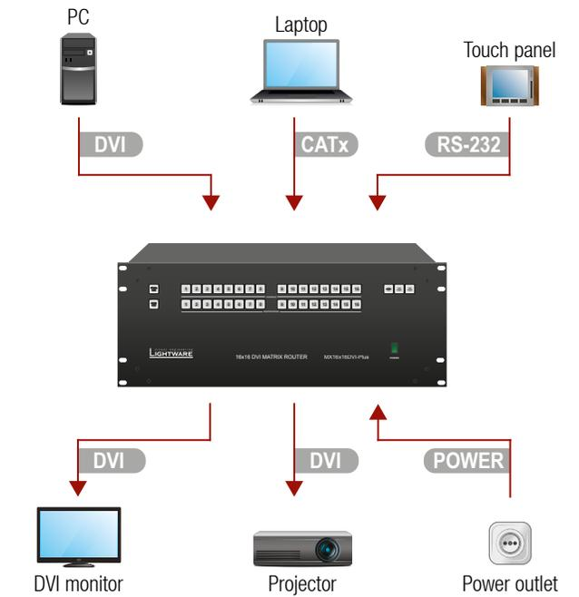
**DVI** Connect the desired sources to the **DVI input ports**.
