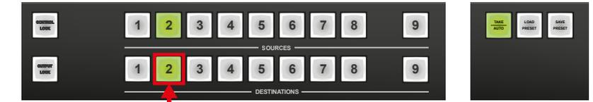
The pressed destination button and the actually connected source button light up green. If no source is connected (the output is muted) no source button will light up.
