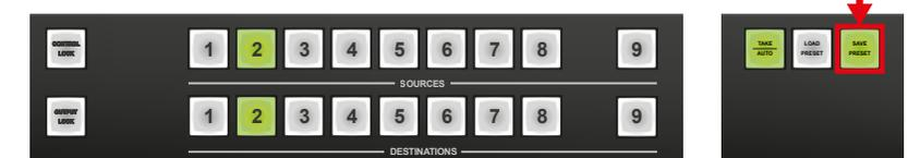
**Step 3.** Press and release a **source** button according to the desired memory address.
