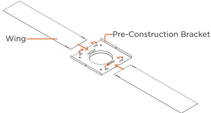
2. Once in place, fold tabs on pre-construction bracket down (x4).
