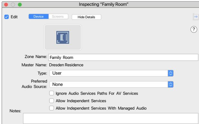
**Allow Independent Services** - Allows more than one service to be active at once. When there is more than one audio endpoint in the zone they could be playing different audio at the same time.
