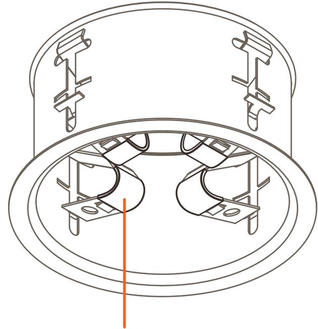
If the ceiling is 5/8" thick or greater remove the rubber friction bands from the springs.
