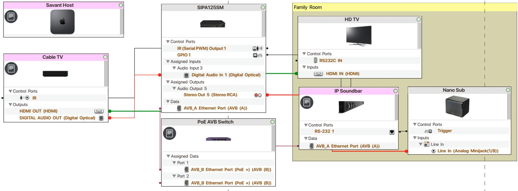
**⚠ IMPORTANT!** The above example shows the analog audio output of a PAV-SIPA125SM used in a speaker group. The analog output of a PAV-SIPA50SM cannot be used in AVB Speaker Grouping.
