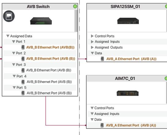
Savant IP Audio device Ethernet ports should be connected to ports on the AVB switch as shown in the example image.
