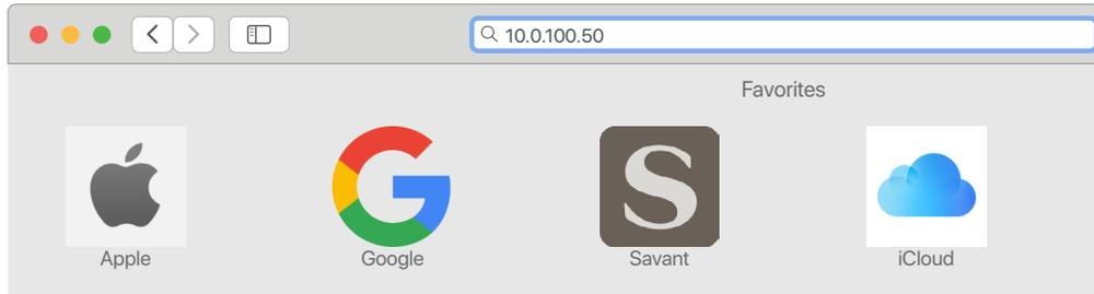
Also the Web UI can also be opened from System Monitor on the Controller Info tab. With the desired IP Audio device selected Click on the IP address listed, this will open the default web browser and connect to the device's web UI.
