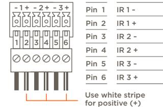
**NOTE:** While not shown in the diagram, IR connections 4 to 6 follow the same wiring as 1 to 3.
