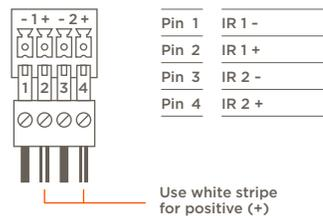
**NOTE:** While not shown in the diagram, IR connections 3 and 4 follow the same wiring as 1 and 2.
