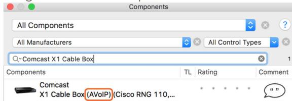
This example supports several model numbers. While searching for devices to add to the configuration if two version appear in the search and the device is going to be controlled by a Video over IP control port use the profile with the AVoIP tag in the profile name. For more information on available profiles see the **Savant IP Video: AV Devices May Require Alternate Profile for IR Control Application Note** on the **Savant Customer Community**.
