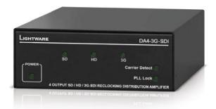
Lightware DA4-3GSDI is a multirate one Input four Output serial distribution amplifier. Input equalization provides compensation of 100 m (3G-SDI) cable loss, while Outputs are reclocked and independently buffered. Front panel LEDs gives a quick information about the DA status: power, data rate and PLL lock status. The unit has a built-in power supply and housed in a metal enclosure for long term reliability and hard environment operation.
