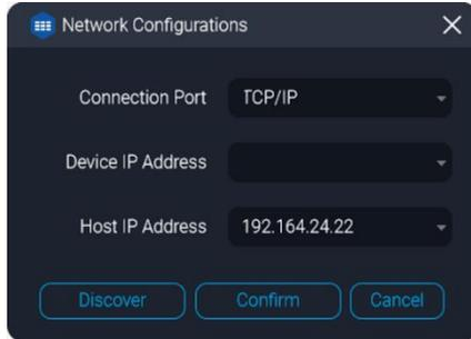
Select the Connection Port: **TCP/IP** or **COM Port**. The default connection is **COM Port**.
