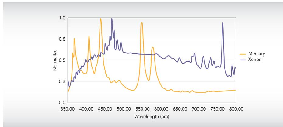
▲ Xenon vs high pressure Mercury lamps
